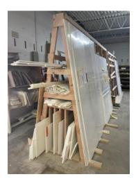
AMI uses A-Frames to store Flat Stock and Wall Panels, placing the largest panel in the back, fully supported, and having each panel finished surface to finished surface and unfinished surface to unfinished surface. The space under the A-Frame can be used to store trim, molding, and smaller flat stock pieces like splashes.
